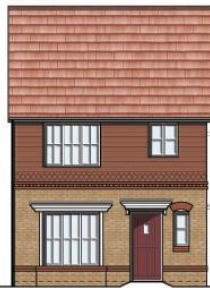
Front Elevation (Tile Hanging) Scale 1:100
