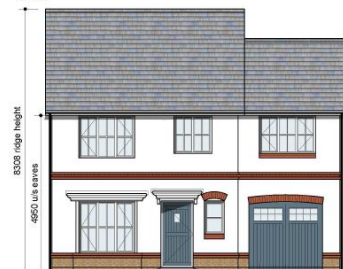
Front Elevation (Tile Hanging) Scale 1:100
